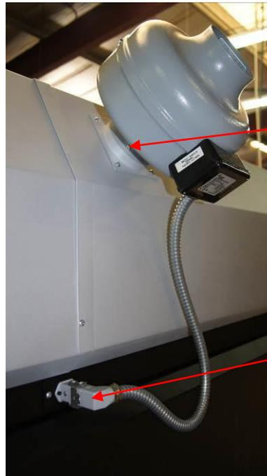
Place the fan on the flange and screw the 3 screws curved M5-12
